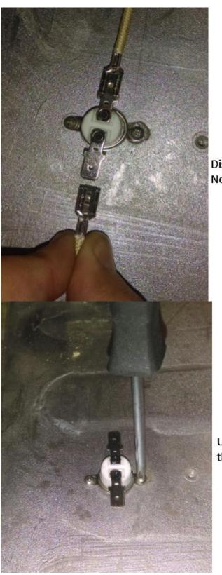
Disconnect both wires from the thermostat disc. Needle-nosed pliers may make this a little easier.
