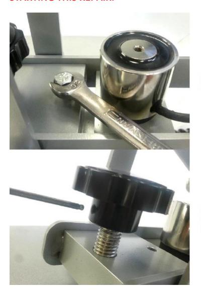
Remove Safety Bolt behind Adjustment Knob using 1/2" Wrench
