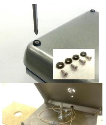
Unscrew 4x #10-24 x 5/8" Screws with Plastic Finishing Washers using #2 Philips Screwdriver
