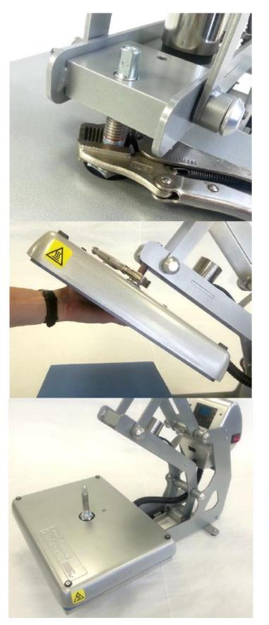
Grip the spindle using Pliers
